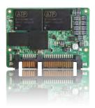
ATP SlimSATA modules offer premium performance and reliability. Advanced Wear Leveling extends usage life; PowerProtector provides hardware-based data protection against power fluctuations and failures; and four mounting holes are available for secure installation against shocks and vibrations, making ATP SlimSATA ideal for business-critical industrial PCs, advanced telecommunications computing architecture, single-board computers, surveillance and security, and networking environments.
