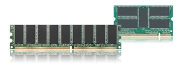
Double Data Rate (DDR), also known as DDR1, is the second generation of Synchronous DRAM (SDRAM). As its name implies, double data rate refers to its ability to read and write data on both the rising and falling of the system clock to achieve nearly twice the bandwidth of single data rate (SDR) SDRAM.
