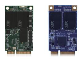
Just roughly the size of a business card, ATP's mSATA SSDs offer up to 512 GB capacity and the same speed and efficiency of SATA. They are designed to fit in systems with space constraints and high-performance requirements such as embedded and networking applications.
